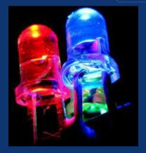
Like all diodes, LEDs create a voltage drop in the circuit, but typically do not add much resistance. LEDs will show up in a schematic as a diode symbol with lightning bolts coming o8 of it, to indicate that it is a glowing diode.
